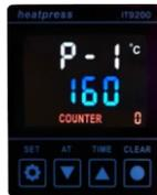
Press the "SET" key into temp. setting mode and the "▲▼" key to set temp.
